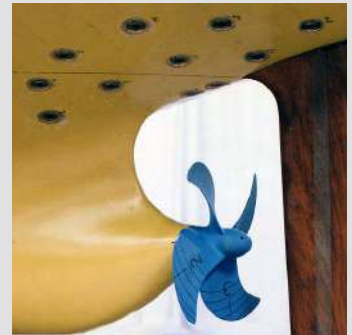
Figure 12: Pressure tabs on a ship's hull, courtesy Mr. Frans Hendrik Lafeber, MARIN
