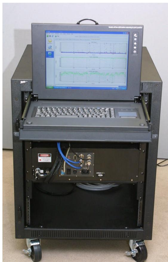
***Artium Technologies, Inc.*** Introduces the **LII200** system, the most advanced laser-induced incandescence instrument available in the market today. Laser-induced incandescence is an optical technique for accurate, non-intrusive, and temporally resolved measurement of soot volume fraction, specific surface area, and primary particle size.
